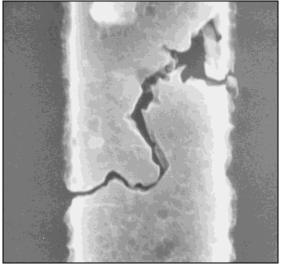
Mass transport of metal-ions in the direction of current flow is a mechanism for interconnection failure. Failure results from the flux divergence of the migrating ions and is accelerated by current density and temperature.
